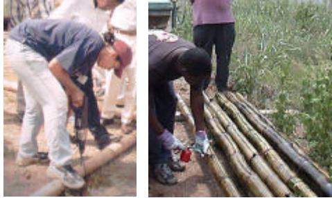
Pictures 1-2 Drilling and Injecting Creosote Oil
