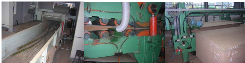
Figure 3.2: Low quality bamboo material used as input (left) for the production (center) of bamboo based MDF (right)
