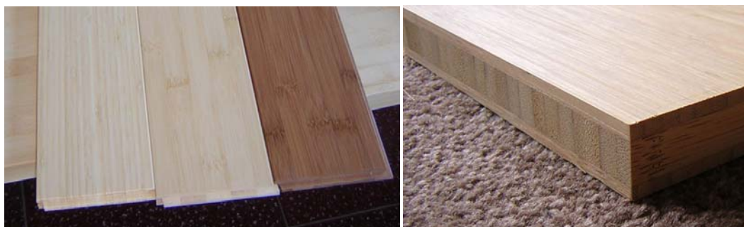
Figure 2.1: Plybamboo is available in various colors, textures and sizes; in the left picture Plybamboo flooring (from left to right: bleached side pressed, bleached plain pressed and carbonized plain pressed) is depicted, in the right picture a sample of a 3-layer carbonized Plybamboo panel is shown
