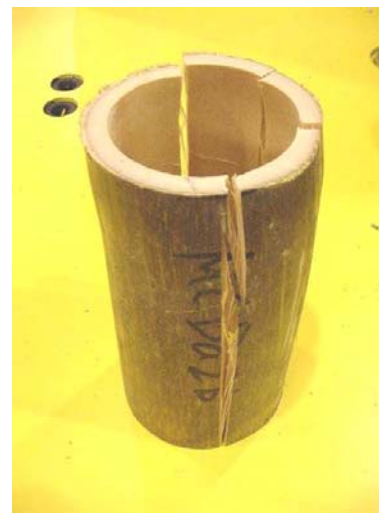
d) Typical failure mode - Splitting
