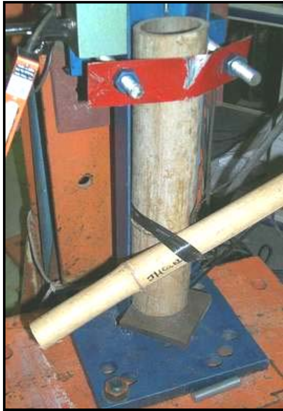
Figure 4.4 Slipping between members
