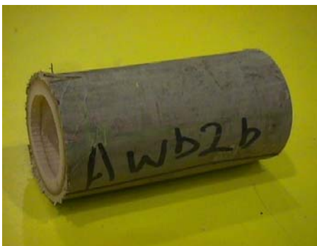
c) Typical failure mode - End bearing
