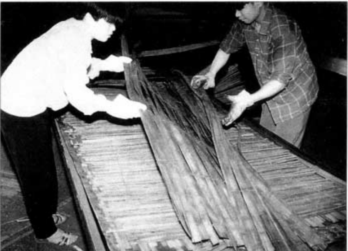
Fig. 12: Laying up strips, wrth alternate layers at rright angles
