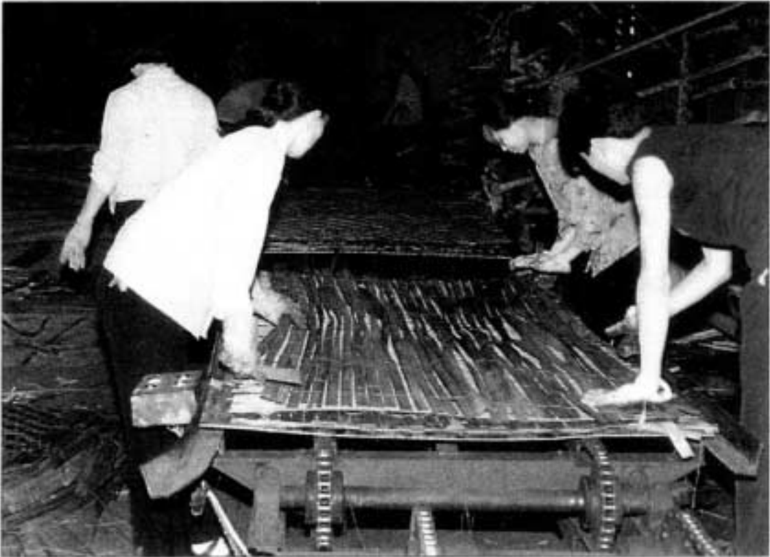
Fig. 11: Laying up strips, with each layer parallel to the other
