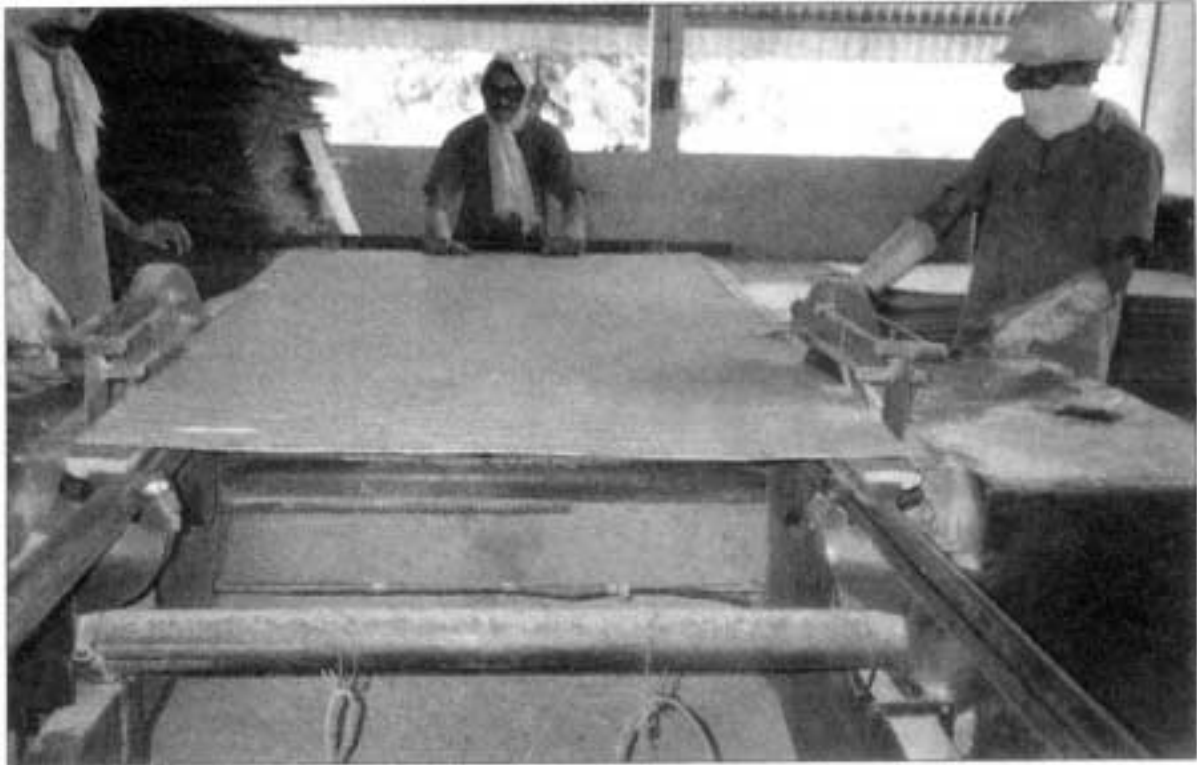
Fig. 5: Trimming of boards
