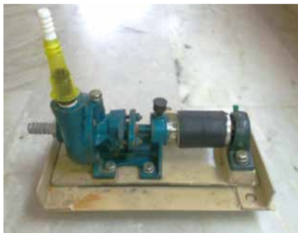
Figure 50: A working prototype of a bicycle driven water pump
