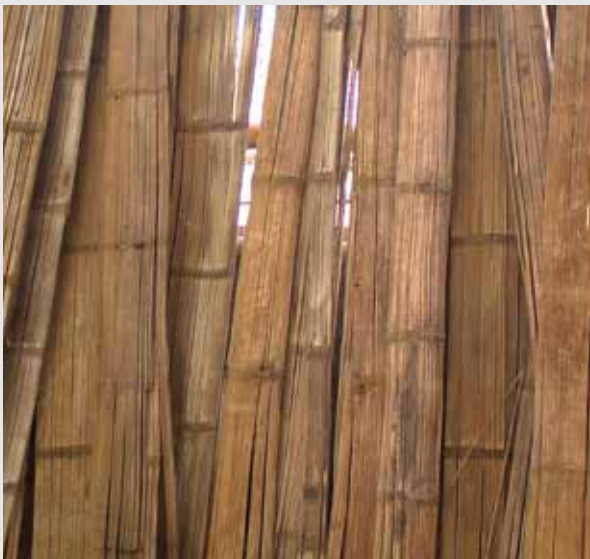
Figure 6: Picture of flattened bamboo
