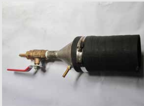
Figure 4: –A closer look at a nozzle connecting bamboo
