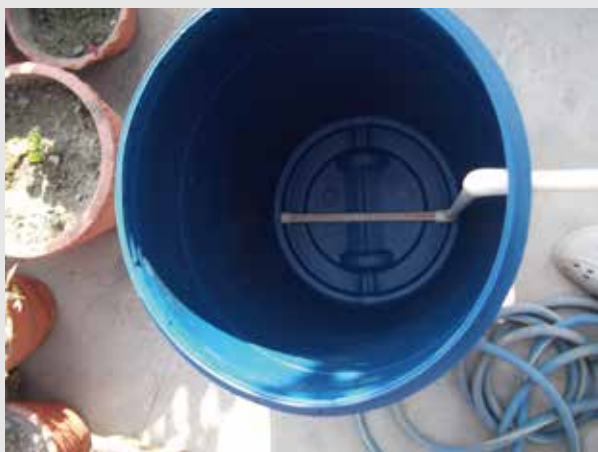
Figure 52: PVC pipe fit to the diameter of the bottom of the biosand filter tank
