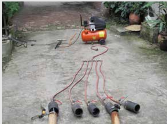
Figure 2: Modified boucherie treatment plant
