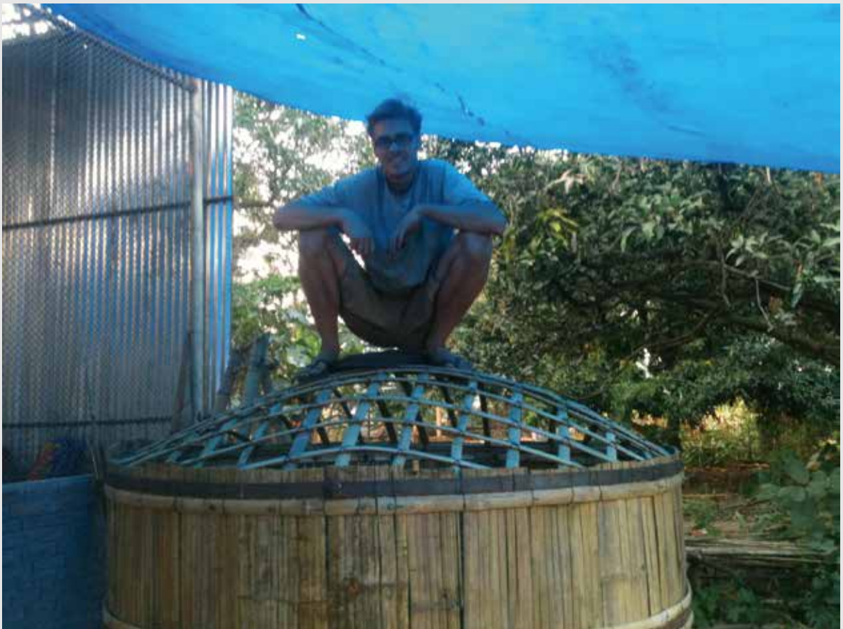
Figure 21: Dome roof with a 90kg load
