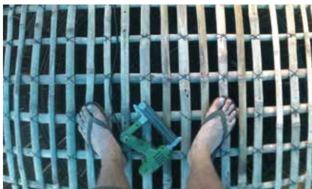
Figure 25: Attaching additional bamboo strips
