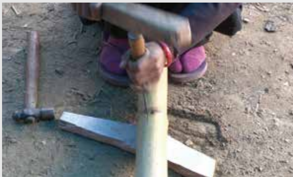
Figure 8: Incision being made at the node
