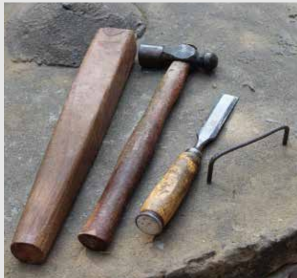
Figure 7: Hammer, mallet and chisel hand tools used to flatten bamboo
