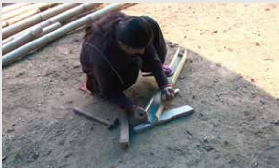
Figure 10: Pulling the bamboo open flat
