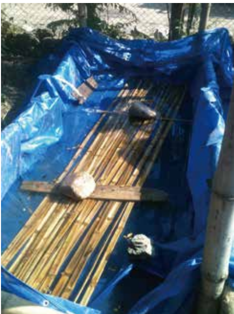
Figure 12: Soaking bamboo strips
