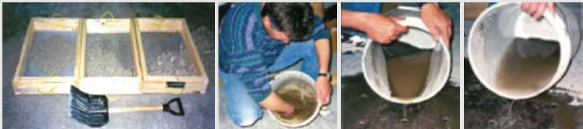
Figure 51: Sieves used for sifting and washing sand and gravel (Source: CAWST, 2008)
