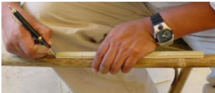
Marked grooves on the culm (triangular mortise)
