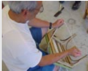
Check the symmetry with a string..
