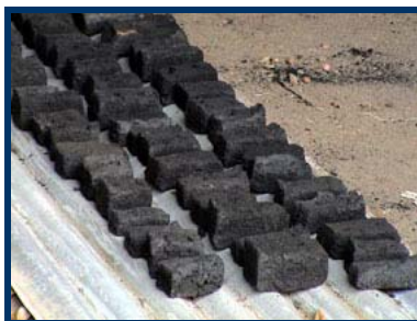
Drying Hand made bamboo briquettes
