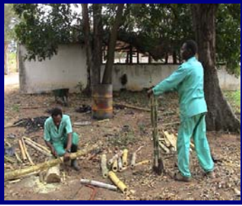
Bamboo being cut and Split
