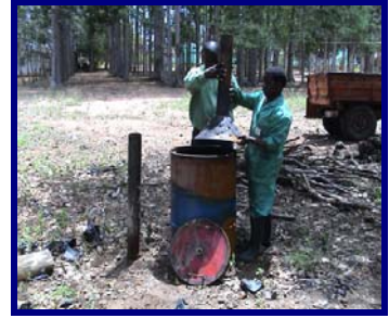
Metal Kiln mounting
