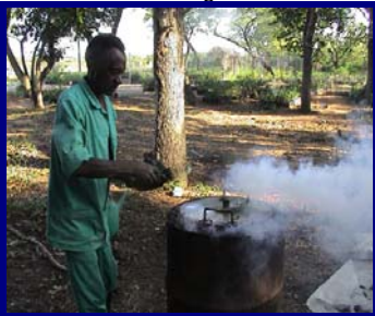
Reducing air intake for carbonisation
