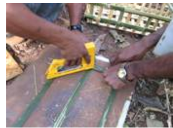
Pneumatic stapling the slivers
