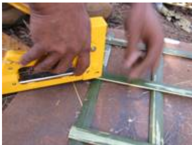
Pneumatic stapling the slivers
