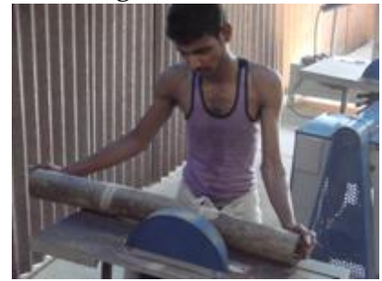
External node removal
