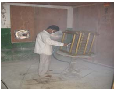
Finishing: spray painting
