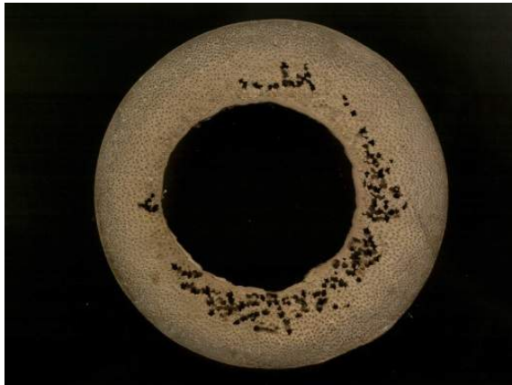
Figure 36: Cross-section through insect-damaged bamboo (Trujillo, 2014)
