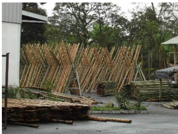
Figure 44: Air drying of bamboo outside, Colombia (Kaminski, 2016)
