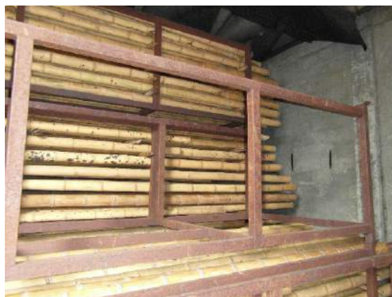
Figure 45: Kiln drying of bamboo, Colombia (Kaminski, 2016)
