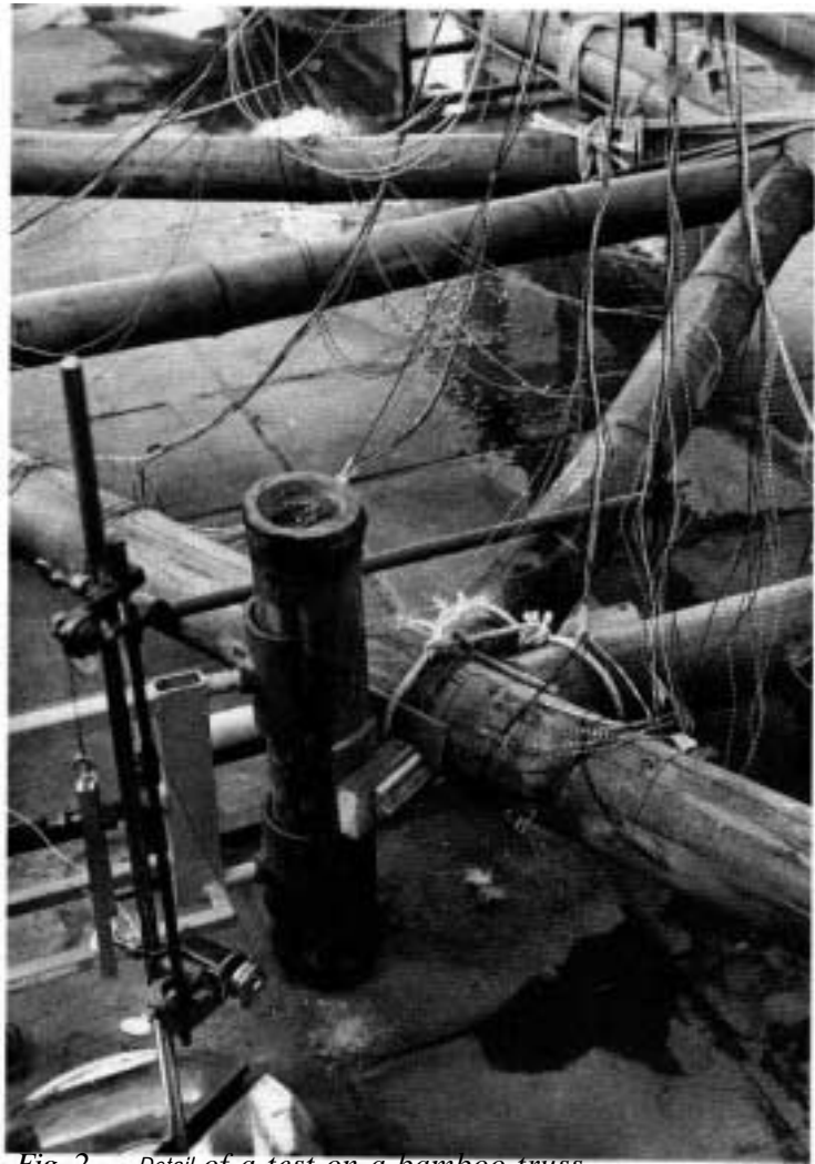
Fig. 2. Detail of a test on a bamboo truss.
