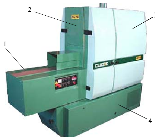
1. Working table 2. Feeding system 3. Sawing unit 4. Base
