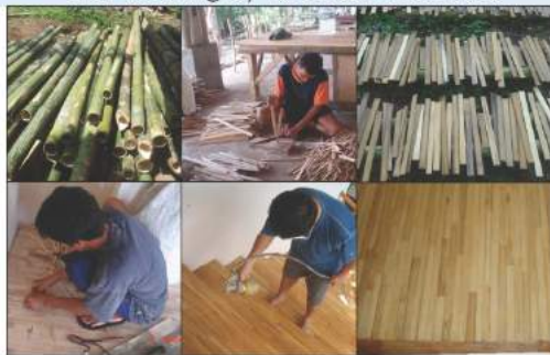
Slat-flooring by rural communities
