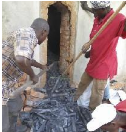
Plate 24: Unloading charcoal with rake collection to prevent contamination
