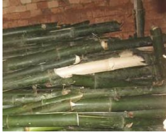
Plate 20: Loaded bamboo culms in a kiln
