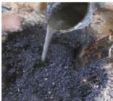
Plate 29: Mixing clay and powdered charcoal with water
