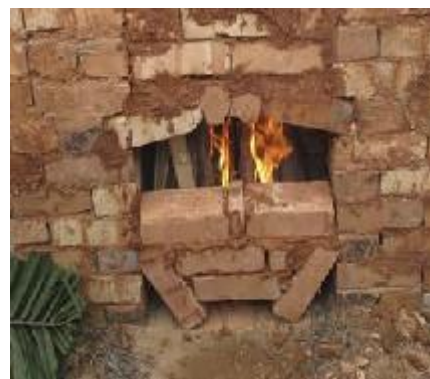
Plate 22: Ignited bamboo firewood in a kiln
