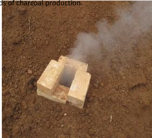
Plate 3: Chimney of a bamboo charcoal kiln
