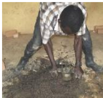
Plate 30: Pressing the mixture to mould the briquette
