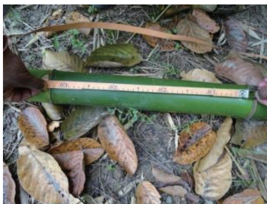
Fig. 2.12: Measuring length of the internode
