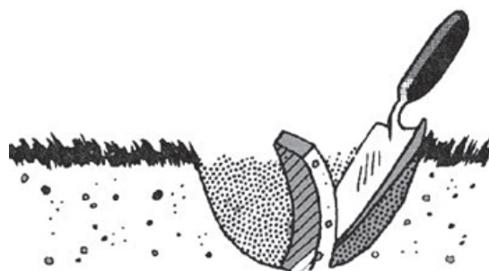
Fig. 4.2: V-shape method for collecting soil samples
