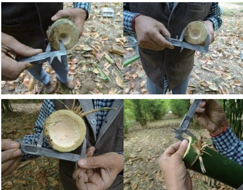
Fig. 2.13: Measuring culm diameter and thickness
