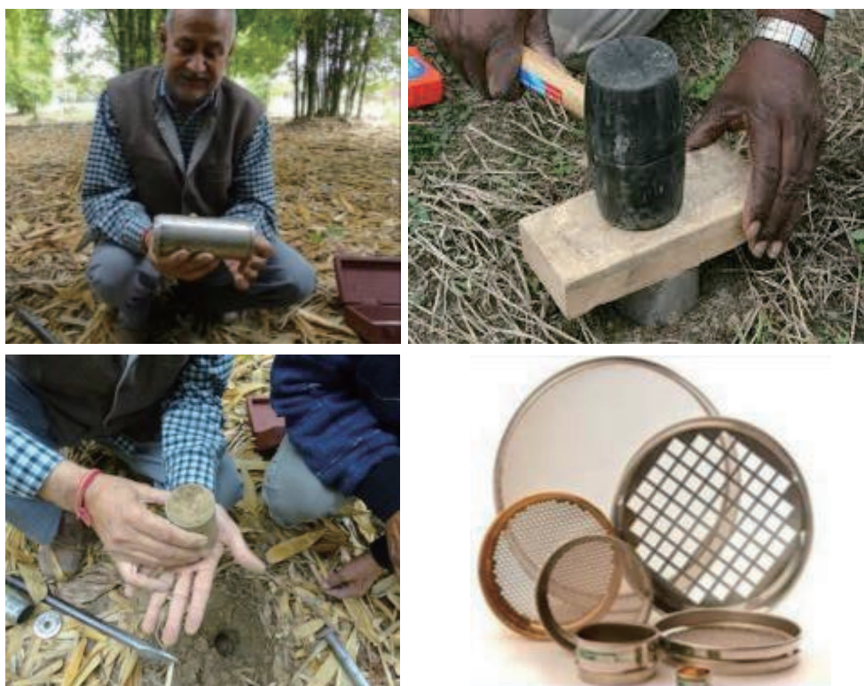
Fig. 2.24: Taking soil samples with core for estimating fine root biomass
