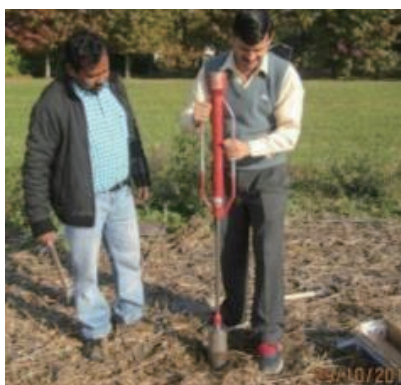
Fig. 4.9: Soil cores being used to collect samples
