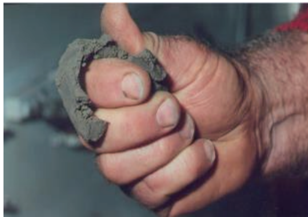
Fig. 4.7: Ribbon formation for determining texture grade
