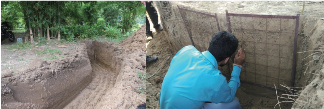
Fig. 2.23: Logarithmic spiral trench and grid arrangement for root study
