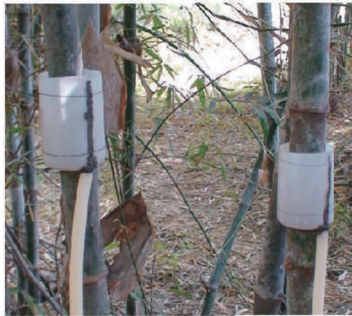
Fig. 3.12: Plastic collars fitted to the bamboo culms to channelise the stemflow
