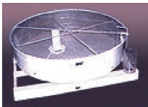
Fig. 3.3: Class A Pan, Standard Evaporimeter
