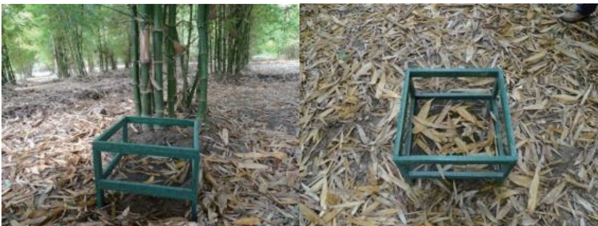
Fig. 2.26: Litter trap for collecting litterfall
