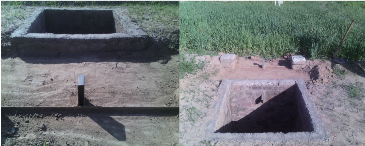
Fig. 3.5: Weir section (front view) of sampler (L) and collection tank (back view) of the sampler
