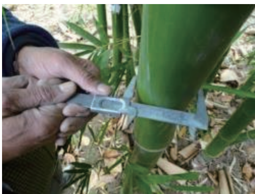
Fig. 2.6: Measuring diameter with the help of caliper
