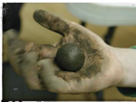
Fig. 4.6: Ball formation for determining soil texture
