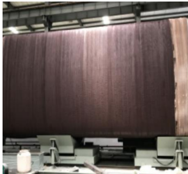
主体缠绕 Main Body Winding
