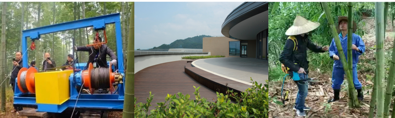
From left to right: A cable towing machine for harvested bamboo poles. Engineered bamboo composite is being used for heavy-duty outdoor installations (Credit: DASSO). Electric bamboo 'scissors' make harvesting quicker and more efficient.
