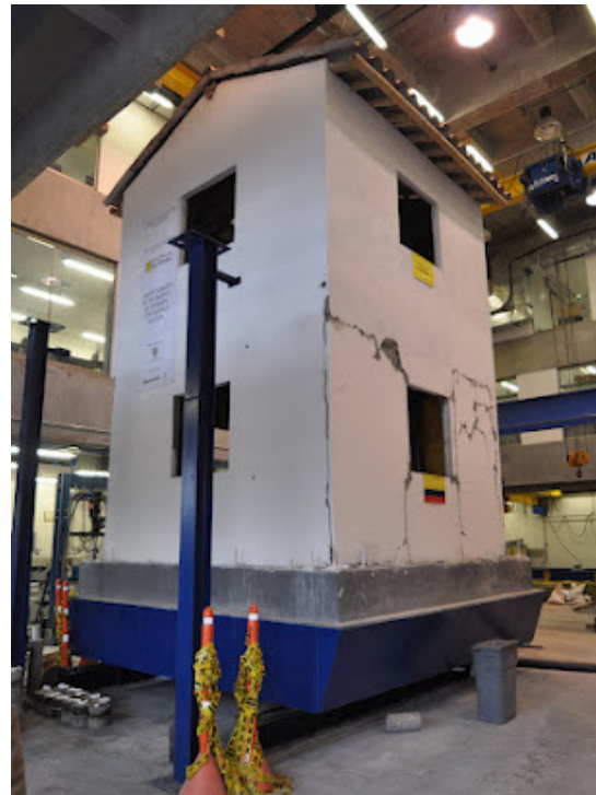
Left: Split bamboo mats nailed onto bamboo frames at 'Bambusa' in Colombia: the first housing project to be designed in accordance with Chapter E.7. Architect: Jaime Mogollón; Engineer: Samuel D. Prieto. Right: Engineered bahareque house on a shake table at Universidad de Los Andes. Its seismic performance was excellent. Credit: David Trujillo.
