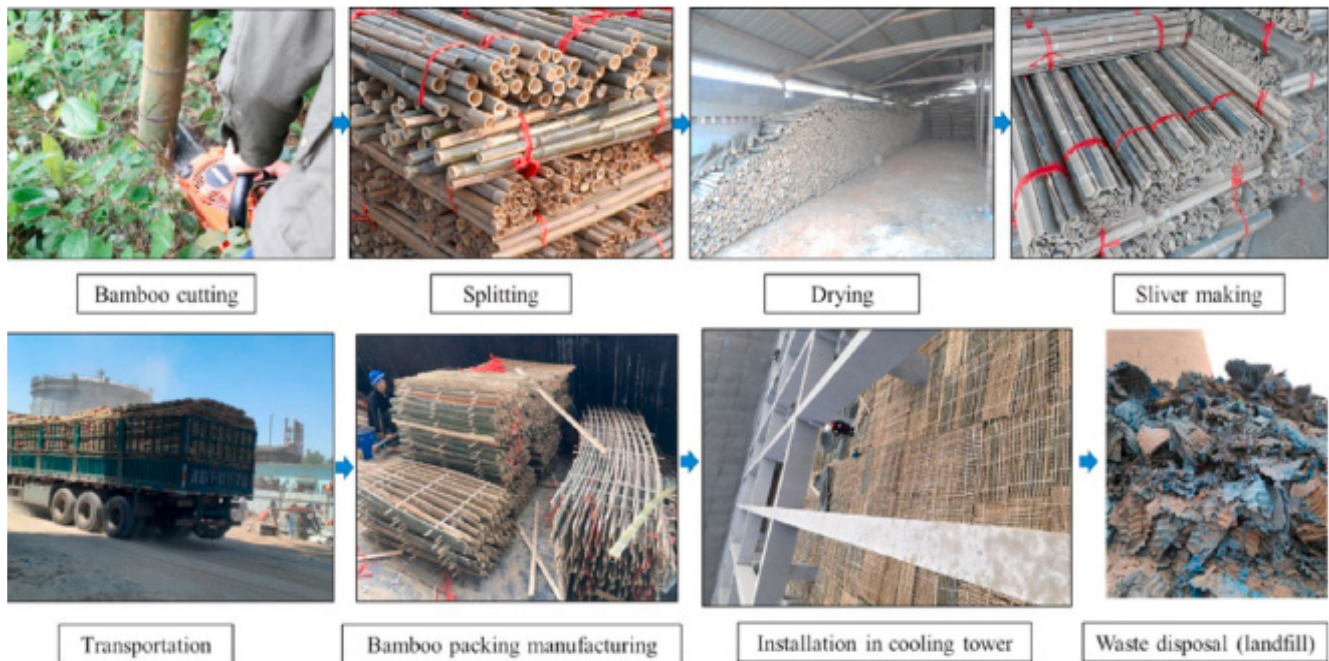
Life-cycle analysis steps for bamboo grid packing in a cooling tower. Credit: Ma Xinxin et al.
