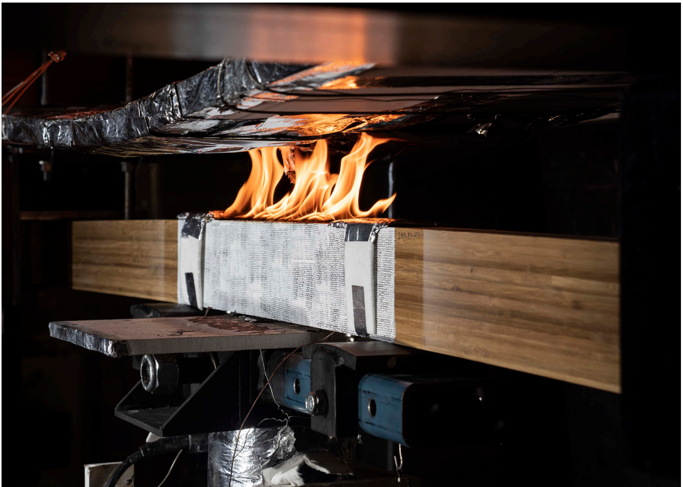
During a fire experiment, laminated bamboo beams are loaded and burned simultaneously. Credit: Genevieve Worrell.
