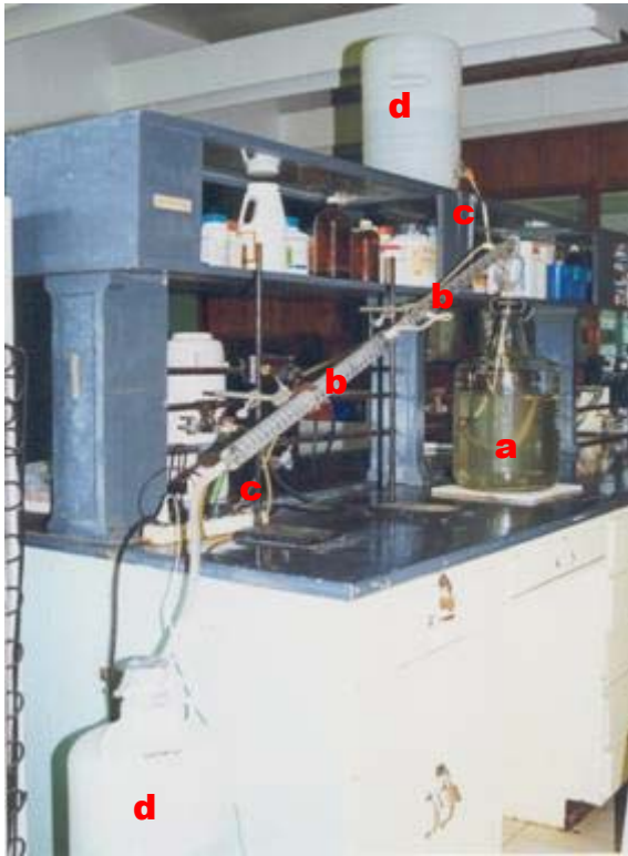
Fig. 2.2. A fabricated distilling unit consisted of (a) 5 gallon glass jar, (b) 2 units condenser, (c) rubber tubings connected to water sources and (d) containers for tap and distilled water (left).
