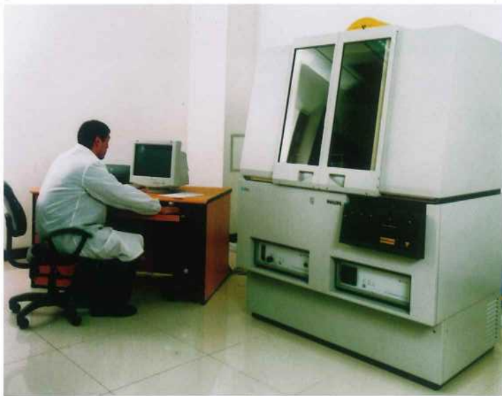
Study on the micro property parameters of bamboo and rattan with the X Ray Diffractometer.
