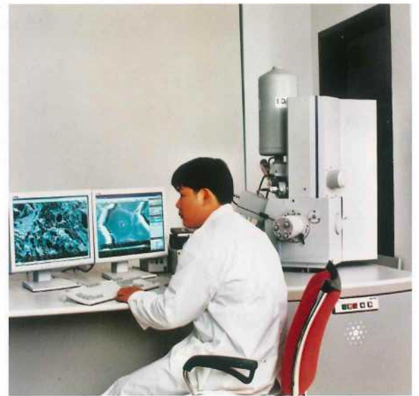
Study on the microstructure of bamboo and rattan with Field Emission Environment Scanning Electron Microscope.
