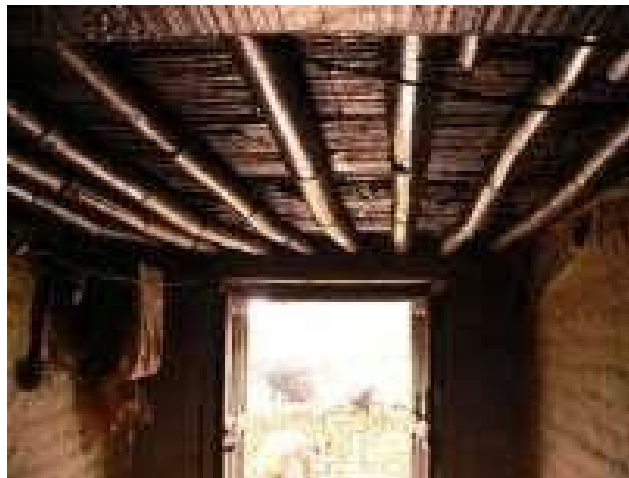
Figure 3. Bamboo culms arranged over a fire source for smoking
