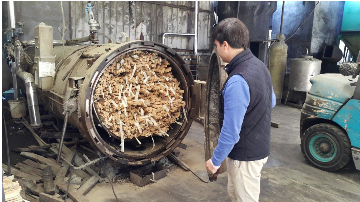
Figure 7. Horizontal arrangement of culms in an electric kiln for drying. (Source: INBAR 2021)
