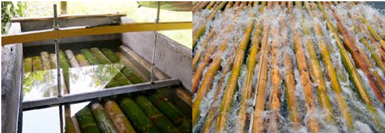
Figure 4. Soaking bamboo in stagnant water (left), and soaking bamboo culms in running water (right) (Source: www.guaduabamboo.com )
