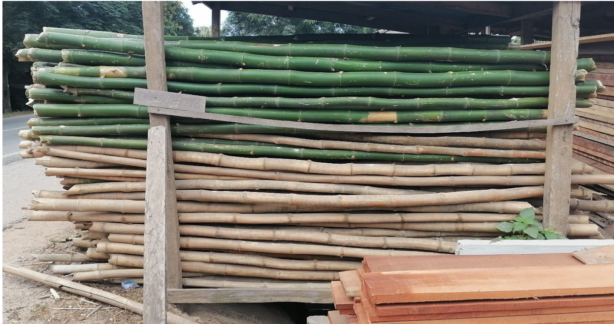
Figure 5. Horizontal stacking of bamboo culms for drying. (Source: INBAR 2021)
