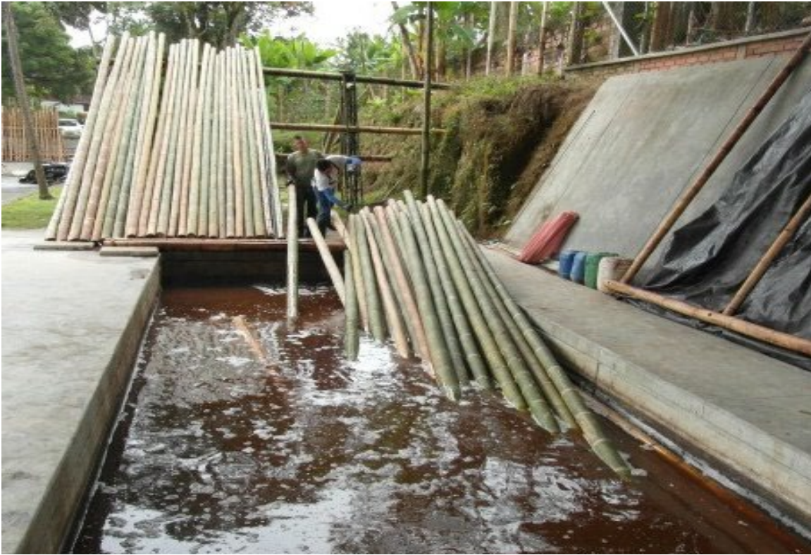
Figure 8. Bamboo culms soaked in a boron-based mixture. (Kaminski et al., 2016)
