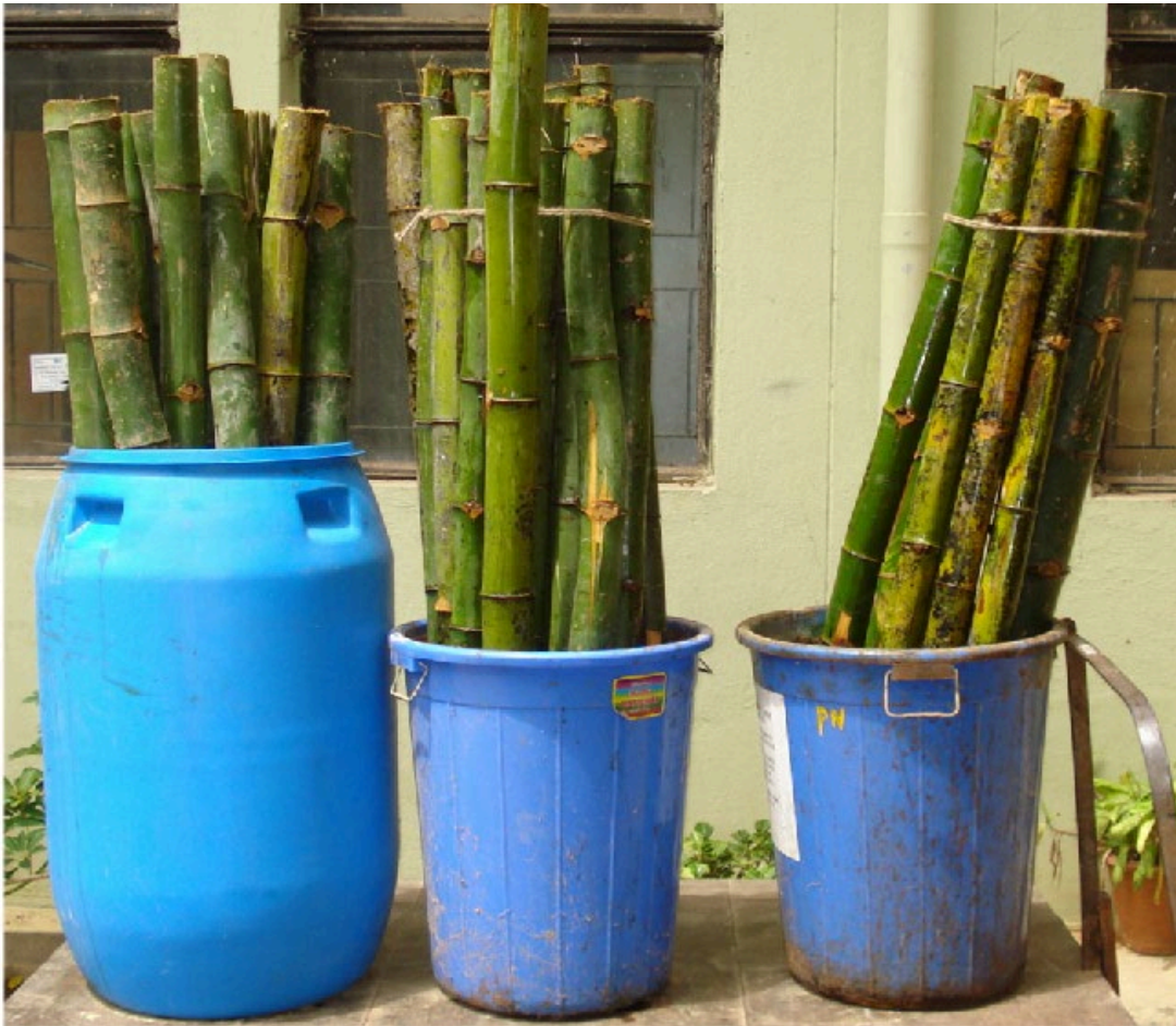
Figure 10. Butt-end of bamboo culms immersed in the treatment solution. (Source: www.semanticscholar.org )
