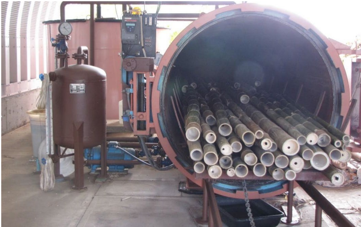
Figure 11. Treatment of bamboo using the pressure method. (Source: www.project.sare.org )
