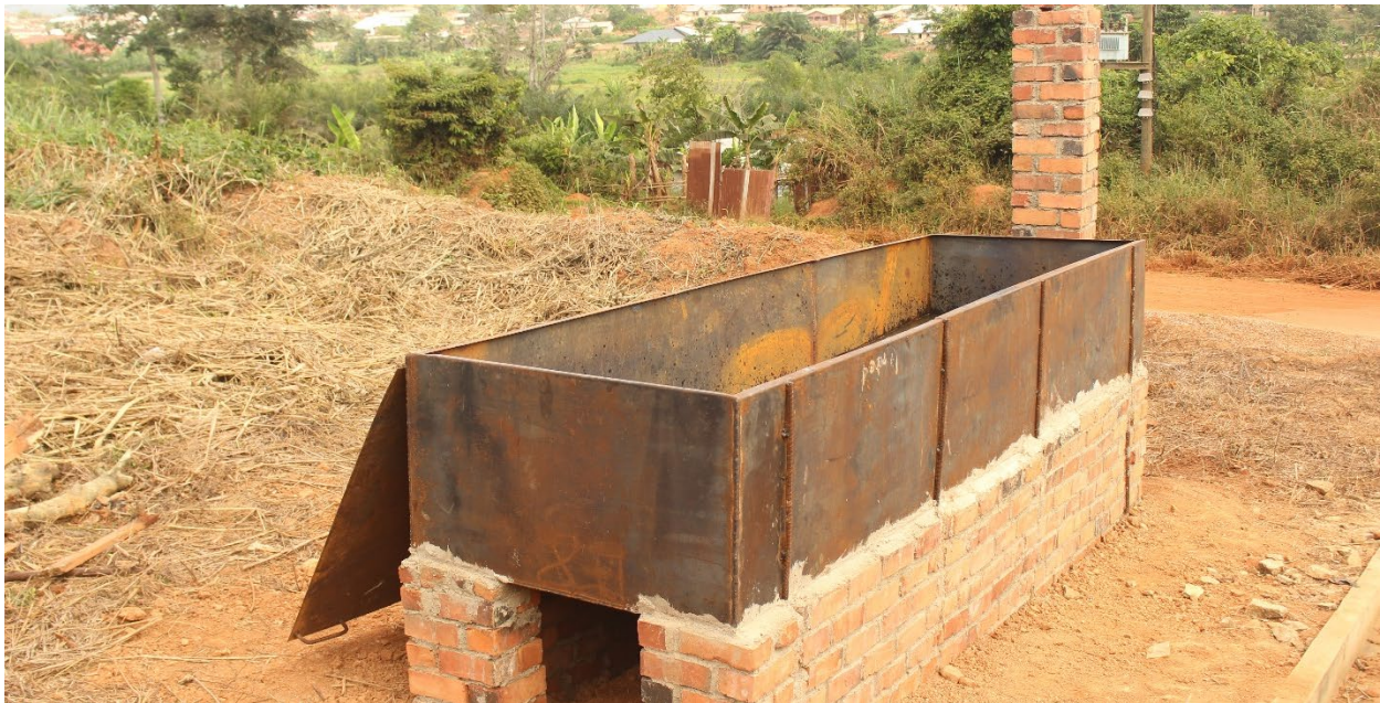
Figure 12. A treatment tank at the Common Production and Training Centre at Obogu, Ghana. (Source: INBAR 2021)
