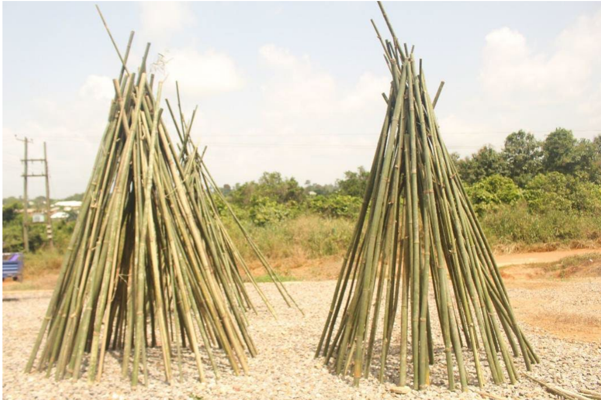
Figure 6. Vertical staking of bamboo culms for air drying. (Source: INBAR 2021)
