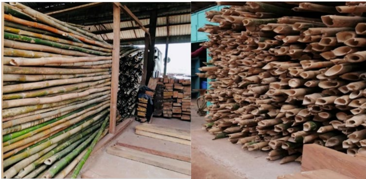
Figure 13. Recommended horizontal stacking of bamboo culms. (Source: INBAR 2021)
