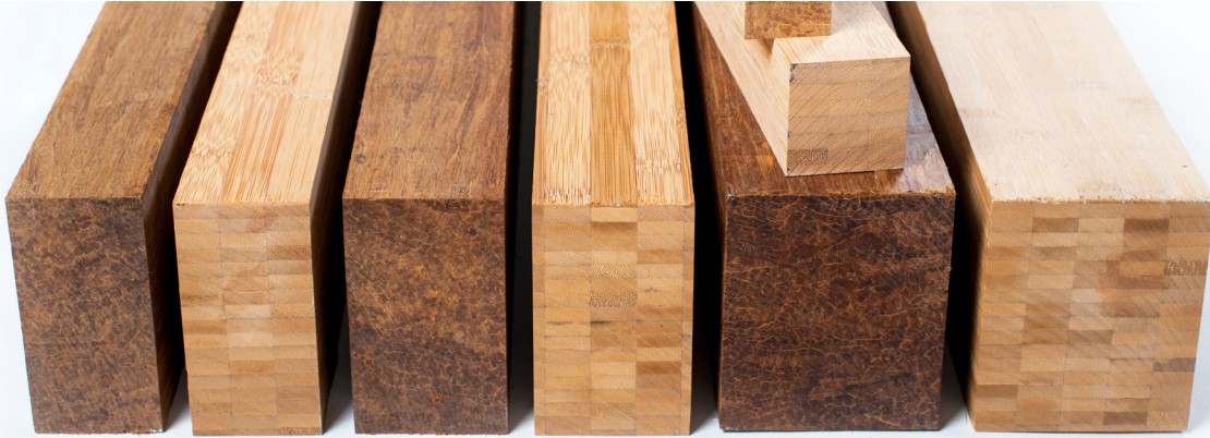
Engineered bamboo beams made from laminated bamboo (yellow color) and densified bamboo (brown color). Credit: MOSO International.
