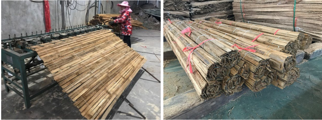
Figure 34: The full-sheet (left) and rolled (right) bamboo fiber bundle curtains made from Ethiopian highland bamboo
