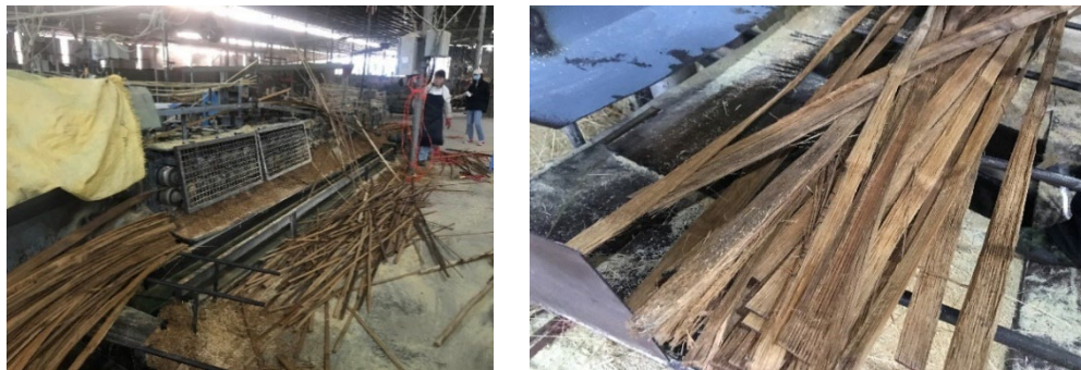
Figure 33: Brooming Ethiopian highland bamboo strips (left) and bamboo fiber bundle strips after brooming (right)
