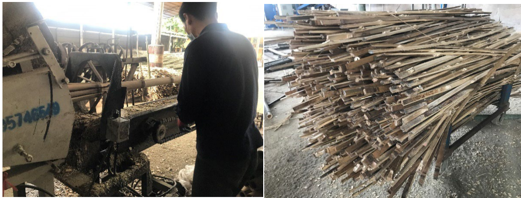
Figure 29: Processing of Ethiopian highland bamboo by splitting machine (left) and highland bamboo strips (right)
