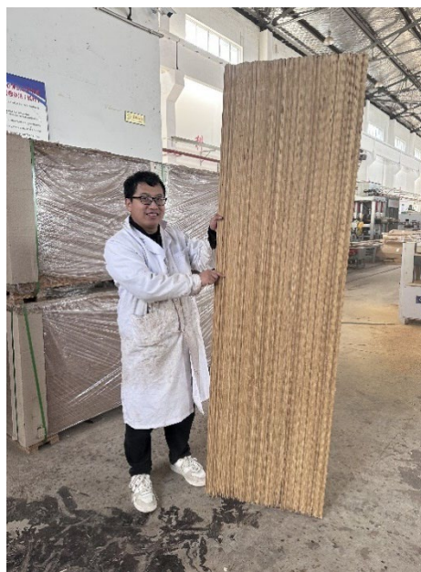
(a) Bamboo laminated sheet
