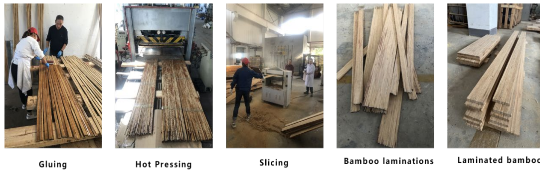
Figure 18: The main produce process for bamboo laminations
