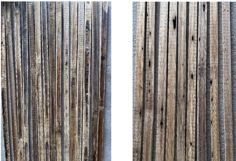
Figure 17: Bamboo strips with inner layers (left) and wormholes (right)
