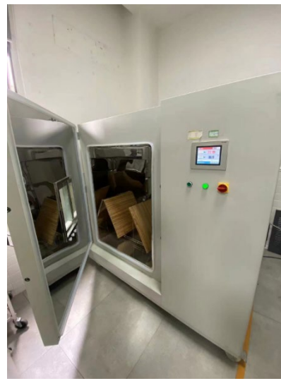
(l) Formaldehyde emission testing
