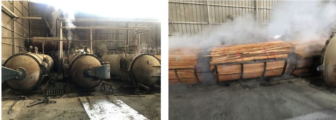
Figure 30: Ethiopian bamboo strips produced by carbonization steaming and softening
