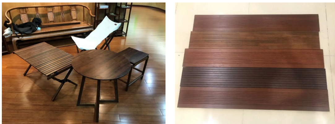
Figure 36: Sample tables and chairs (left), outdoor reassembled flooring (right) fabricated from layers of African highland bamboo bundle laminated composites.
