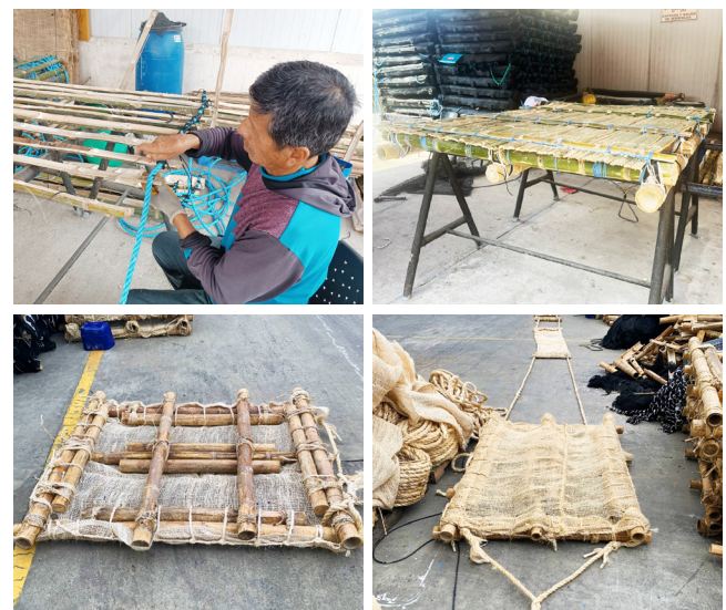
Building bamboo frames for FADs. Credit: INBAR
