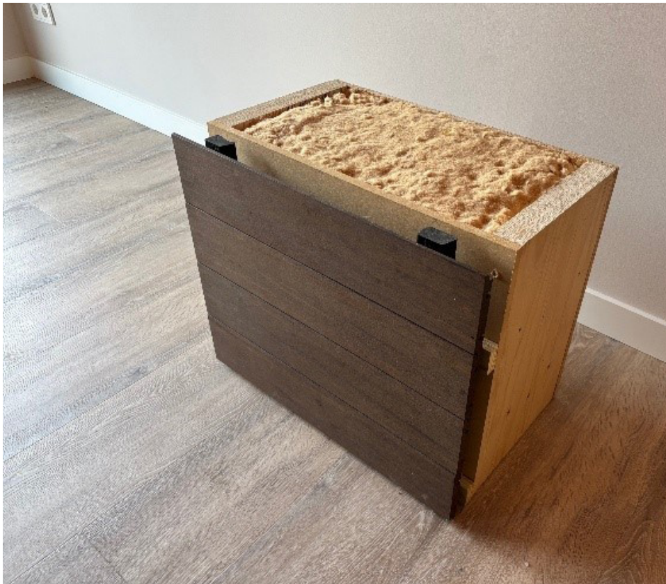
Left: Structural shell of cross-laminated timber and timber framing, wood-fiber insulation and thermally modified bamboo cladding.
