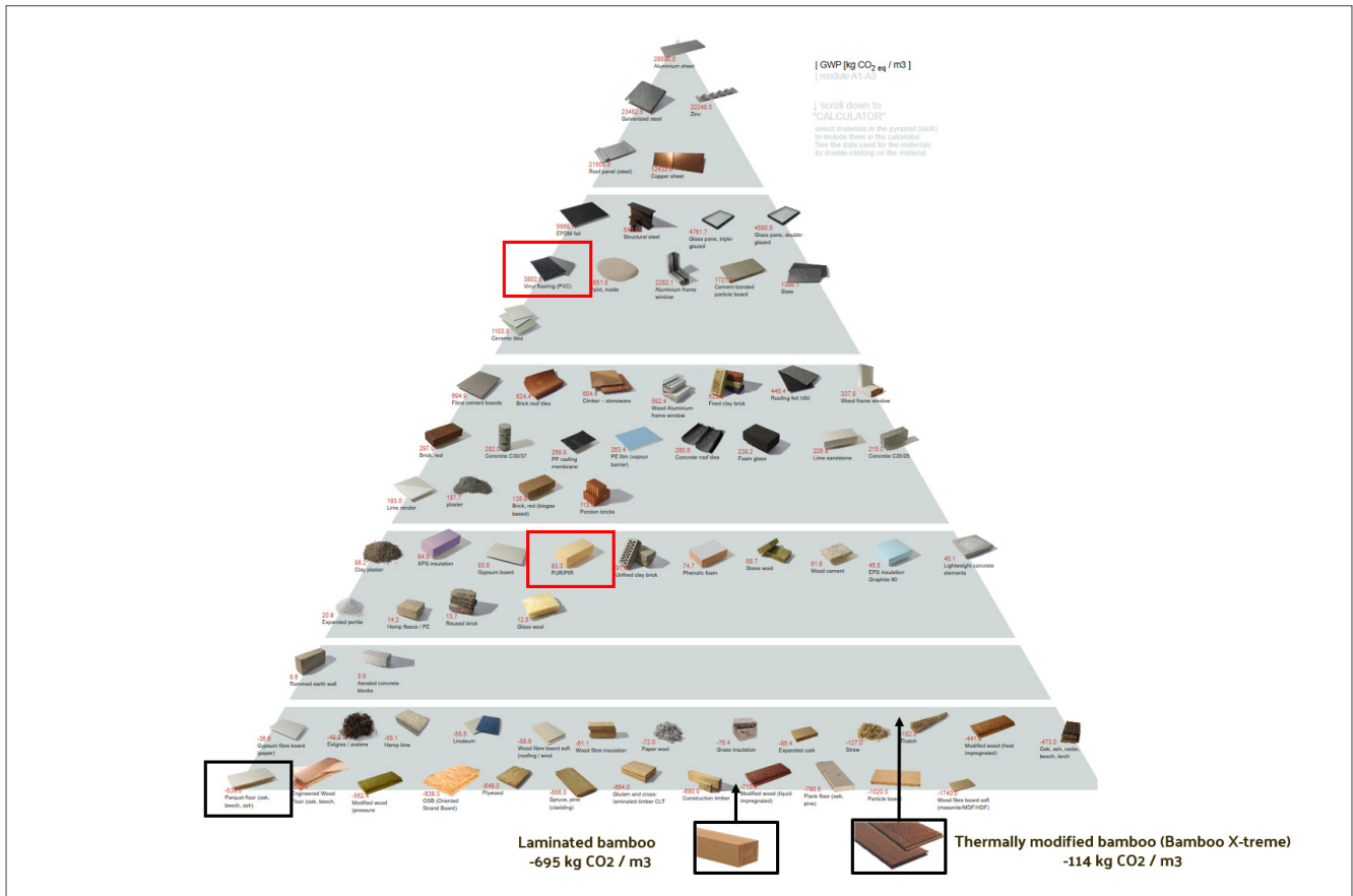
The CO 2 pyramid shows cradle-to-gate emissions per m 3 of building material, based on recent EPDs. Bamboo values are derived from publicly available EPDs for engineered bamboo. Credit: MOSO Bamboo Products.
